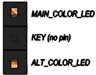
Figure 15 Alternate Power LED header
