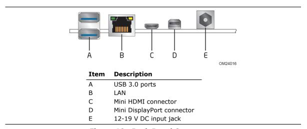
**Figure 10. Back Panel Connectors**
