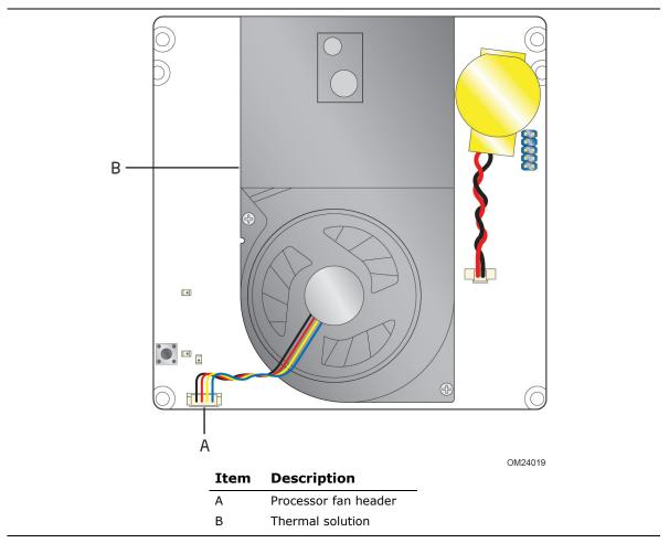
Figure 7. Thermal Solution and Fan Header
