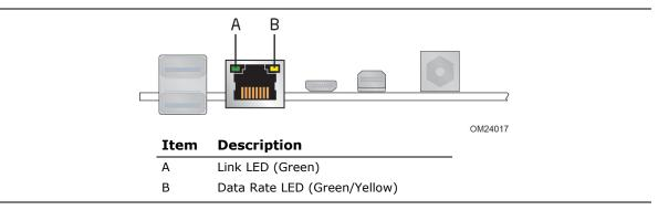
Figure 6. LAN Connector LED Locations
