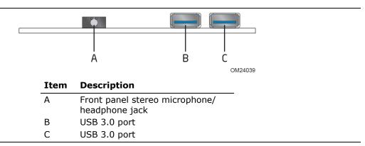
**Figure 9. Front Panel Connectors**
