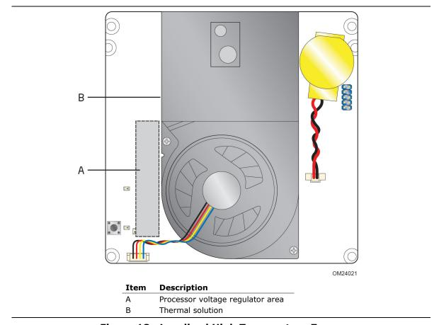
Figure 18. Localized High Temperature Zones
