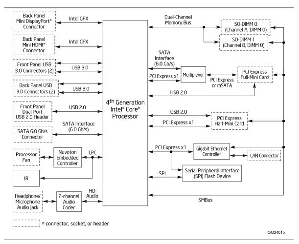
Figure 3. Block Diagram
