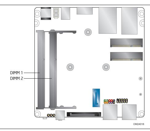
Figure 4. Memory Channel and SO-DIMM Configuration
