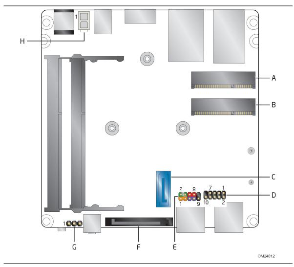
Figure 12. Connectors and Headers (Bottom)
