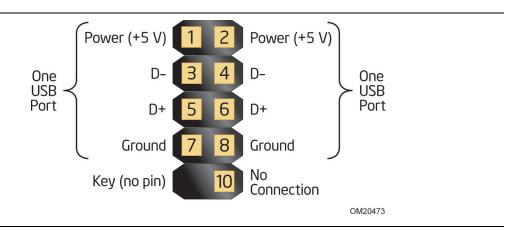
Figure 14. Connection Diagram for Internal USB 2.0 Dual-Port Header (2.0 mm Pitch)
